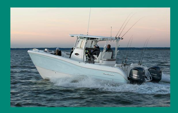
LOA: **29' 1"** Beam: **9' 6"** Fuel Capacity: **233 gal (2 x 116.5)** Dry Weight w/ Power (Approx): **8,500 lbs (w/ twin 300's)** Hull Draft: **15"**
