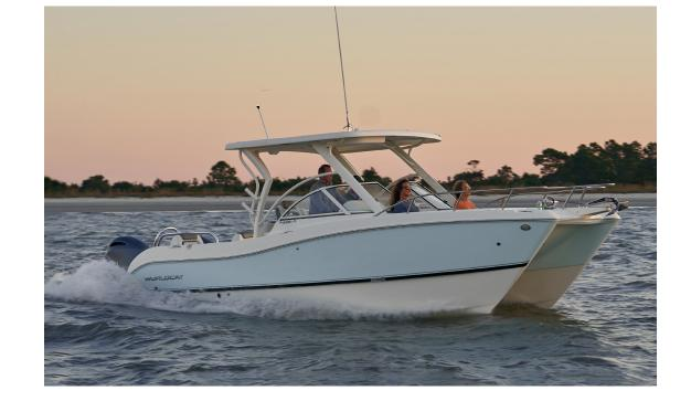
LOA: 26'0" Beam: 8'6" Fuel Capacity: 186 gal (2 x 93 gal) Dry Weight w/ Power (Approx.): 6,600 lbs w/ twin 150's Hull Draft: 12"
