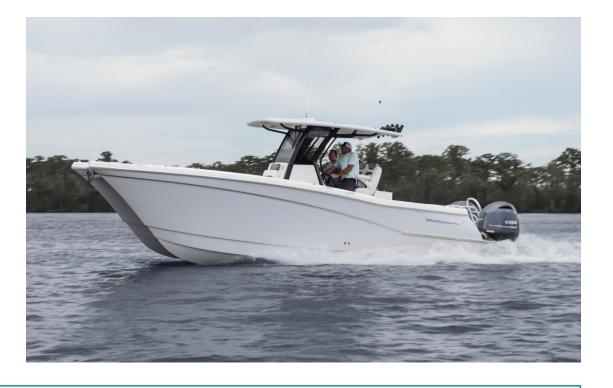
LOA: 27' 6" Beam: 9' 2" Fuel Capacity: 220 gal (2 x 110 gal) Dry Weight w/ Power (Approx): 7,300 lbs (w/ twin 200's) Hull Draft: 14"
